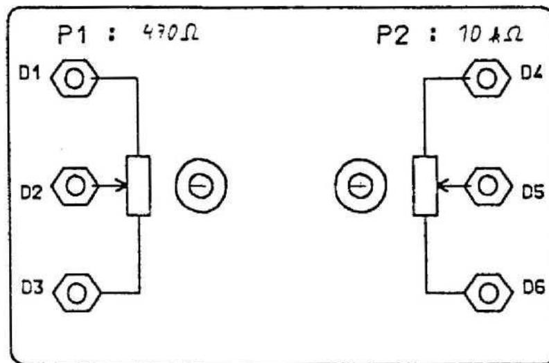
Fig.6 Modul Potentiometer
