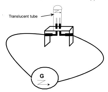
A tube of about 5 ml in unbreakable plastic is filled with a stoechiometric mixture of hydrogen and oxygen (see electrolysis tank). Put it on a multifunction support, the mixture reacts to a spark.
