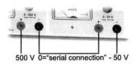
500 V .... 0 .... - 50 V DC outputs when connected in serial. Outputs are floating with respect to ground. Caution: Do not connect any high voltages between any of the outputs and chassis/ground/earth!!! - or the internal transformer will be permanently damaged.
