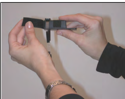
Figure 2b: Fastening the Velcro over the Photogate
