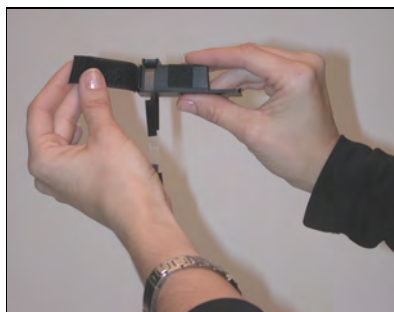
Figure 3b: Fastening the Velcro over the Photogate
