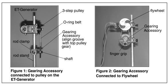
the rod clamp can be loosened to move the Gearing Accessory horizontally for alignment with another pulley groove, etc. For load studies, a hanging mass on a thread can be attached to the shaft on the gear pulley. For suggested experiments and applications with the ET-8775 Gearing Accessory, see the manual provided with the ET-8771 Energy Transfer - Generator. Also see the instruction sheet provided with the ET-8773 Flywheel Accessory.
