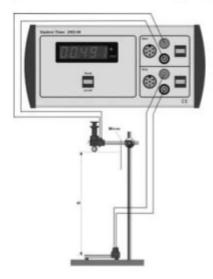
Using this setup the student timer is started when the ball is released from the release mechanism, and the counting is stopped when the ball strikes the switch plate.
