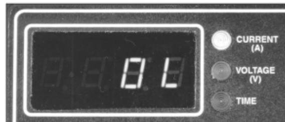
Display shows current Over Load
