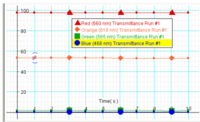
Sample data: transmittance of red, orange, green and blue light through a red solution.
